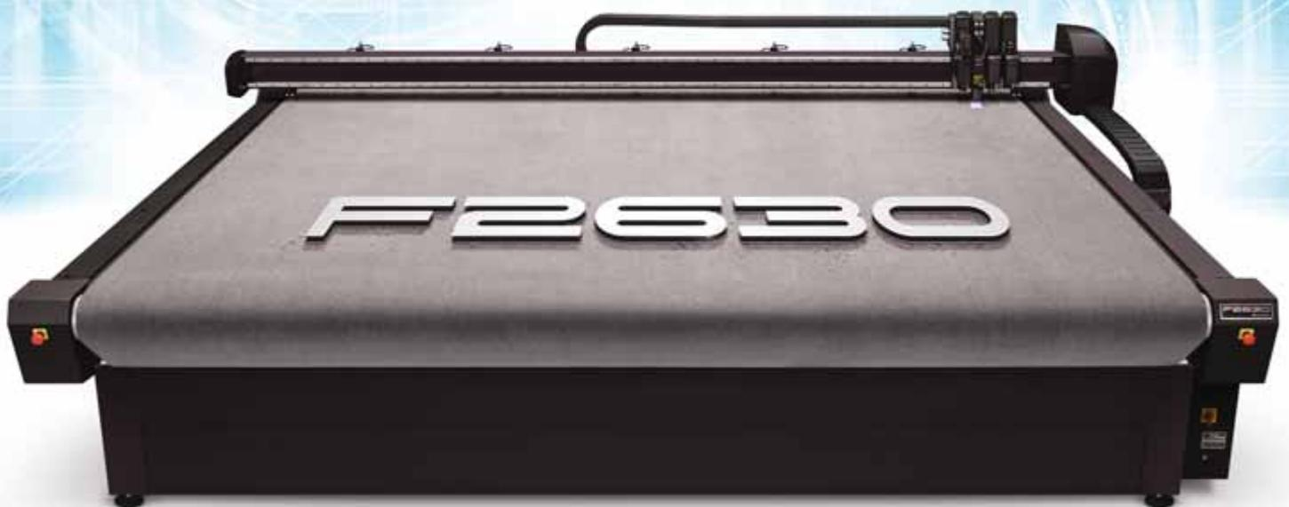
Introducing the new F2630 Grand Format flatbed cutting and finishing system from Summa. The latest addition to the F Series is now available in a size designed to expand your capabilities and dramatically increase productivity. With a cutting area of 265cm X 305cm, the F2630 now brings affordable market potential to the world of large format cutting.
